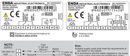
Fuse should be connected Cable size: 1,5mm<sup>2</sup>
