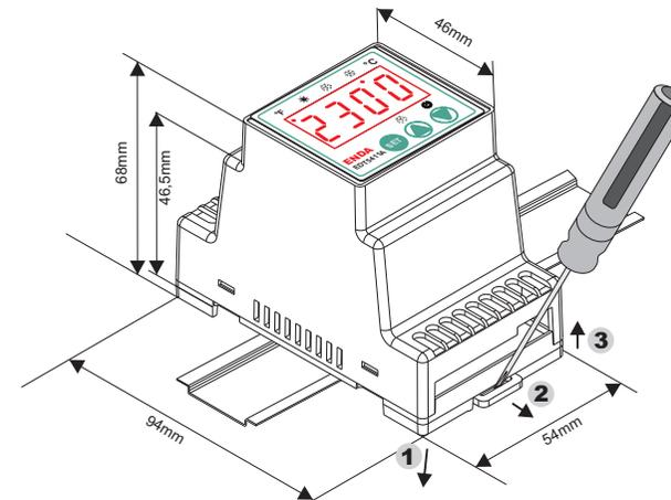
To mounting the device to the panel ; Push the device in direction 1, the rails provide the key to keeping the rail.
