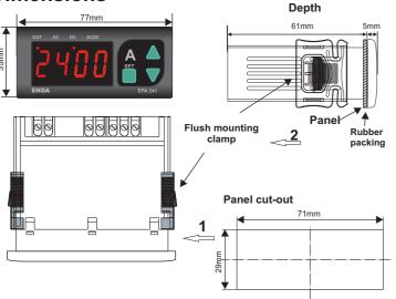
To remove the device from panel:
