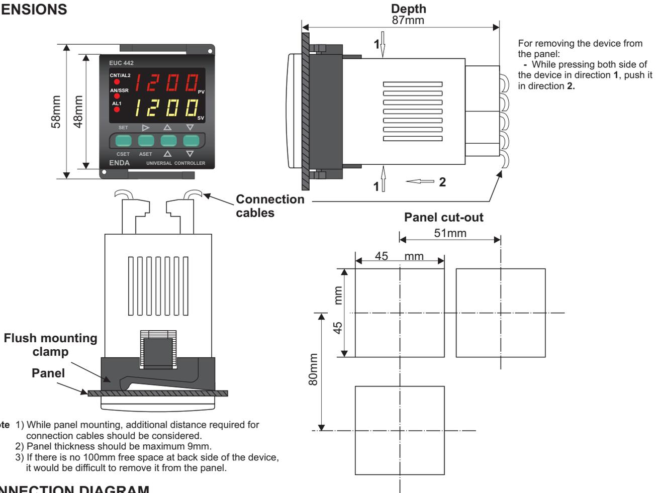
For removing the device from the panel:
