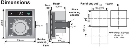
For removing mounting clamps: Push out the flush-mounting clamp in direction 1 as shown in the figure above. Then, pull out the clamp in direction 2. If there is no 60mm free space at back side of the device, it would be difficult to remove it from the panel
