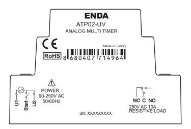
ENDA ATP02 Series timers are rail mounted devices. Make sure that the device is used only for intended purpose. The shielding must be grounded on the instrument side. During an installation, all of the cables that are connected to the device must be free of energy. The device must be protected against
